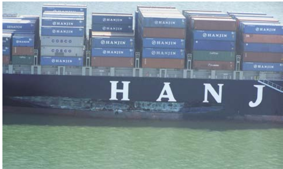
Right: The container ship Cosco Busan leaked oil into the bay from a hole in its hull.
